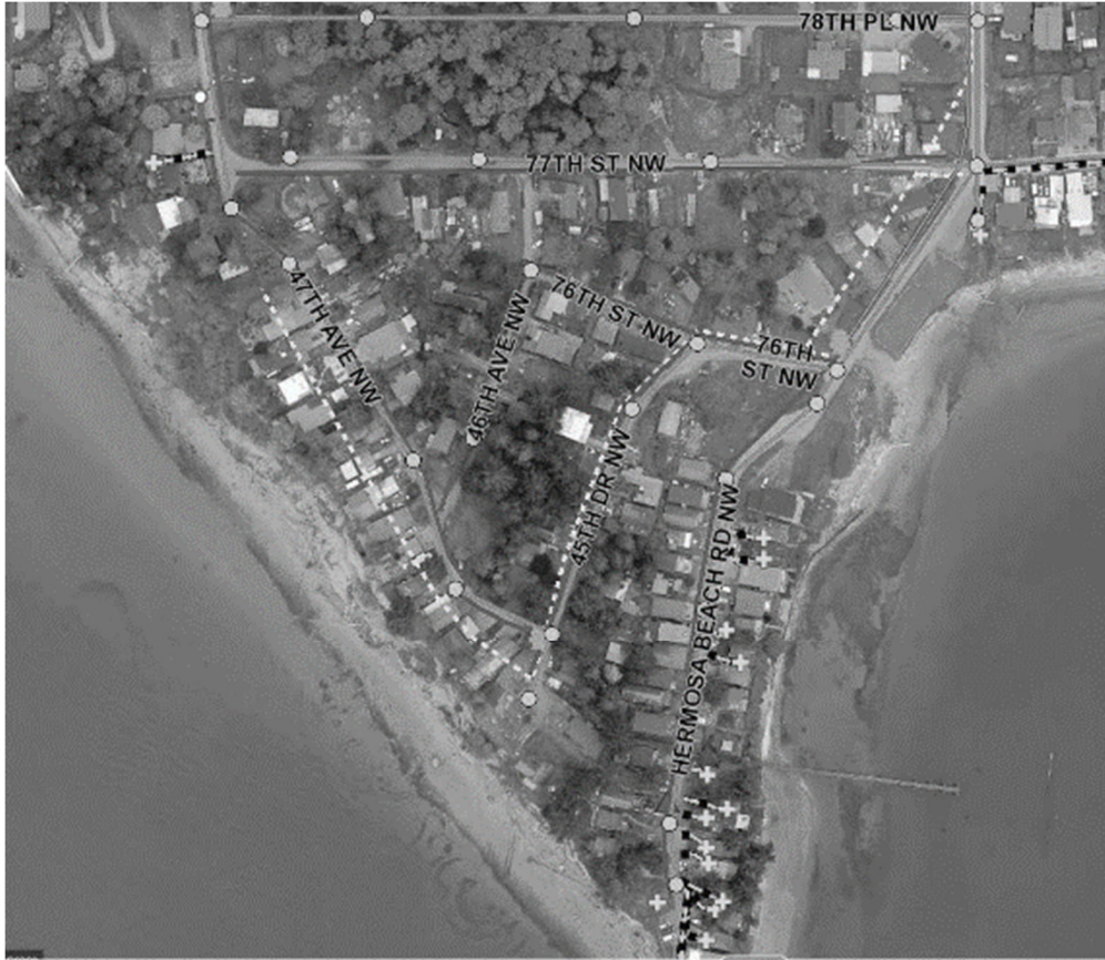
Figure 1c. Hermosa Beach Road, approximately 1,200 linear feet of 6-inch PVC and 78th Place NW 1,250 linear feet of 6-inch PVC.
