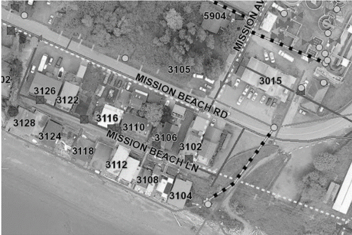
Figure 1a. Mission Beach Road and Mission Beach Lane, approximately 1,175 linear feet of 6-inch ductile iron or PVC.
