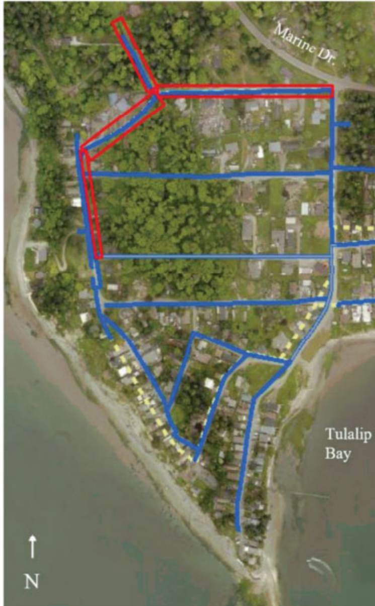
Figure 2. Water mains in Hermosa Beach and Fryberg Estates, lined in blue. Water mains outlined in blue with grey centers are AC. Water mains boxed in red have already been replaced with PVC. Approximately 10,000 linear feet of 6-inch PVC.
