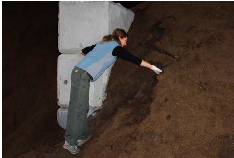
Figure 15. Sampling composted AD manure solids.
